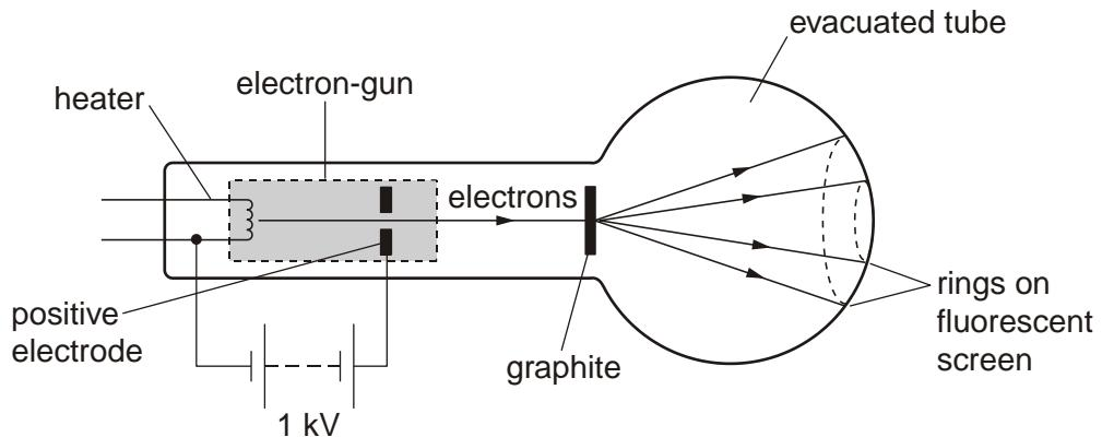
The electrons are accelerated to high speeds by the electron-gun. These high speed electrons pass through a thin layer of graphite (carbon atoms) and emerge to produce rings on the fluorescent screen.
